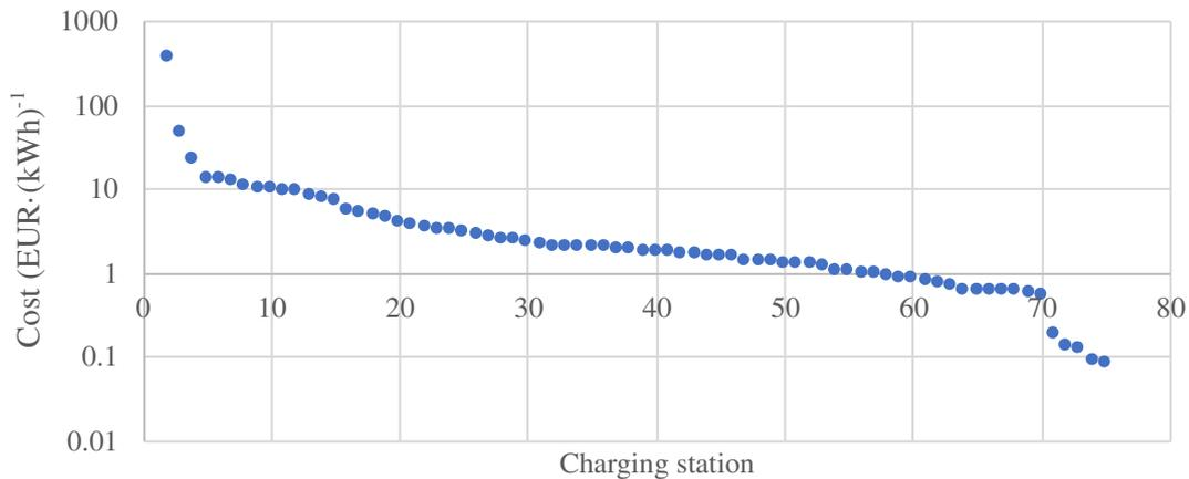
**Fig. 1. Average cost of transmission and distribution per kWh charged in Latvian national fast charging network**
